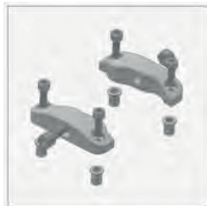
Fastening of frame sections for units of sizes greater than 10 (Fig.. 20)
